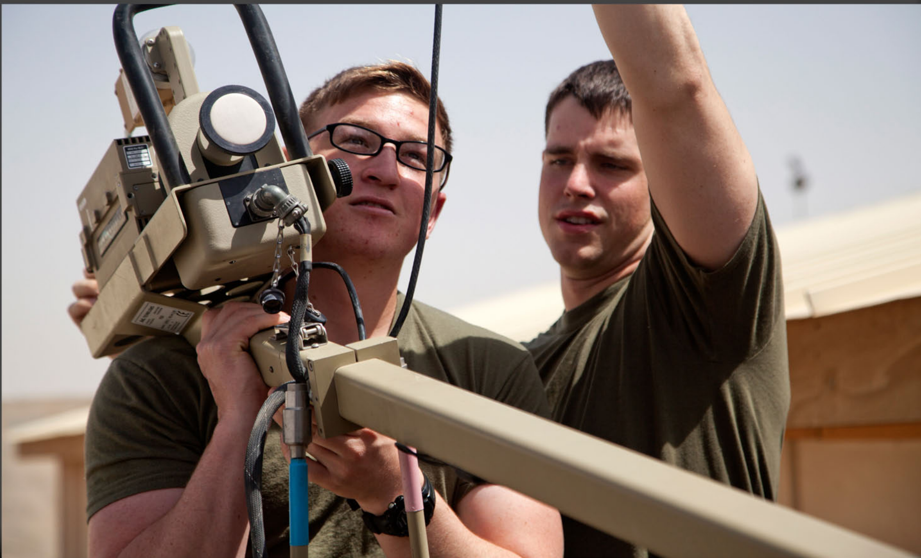
U.S. Marine Corps Lance Cpl. Zachary Schaible, left, and Cpl. Andrew Sanders, assigned to Headquarters Company, Regimental Combat Team 7, set up Secure Internet Protocol and Non-secure Internet Protocol Router Access Point (SNAP) satellite communications system on Camp Leatherneck, Helmand province, Afghanistan, April 24, 2013.
